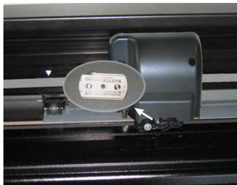
FIG 1-35 RAZOR BLADE FOR AUTOMATIC SEPARATION OF MEDIA
