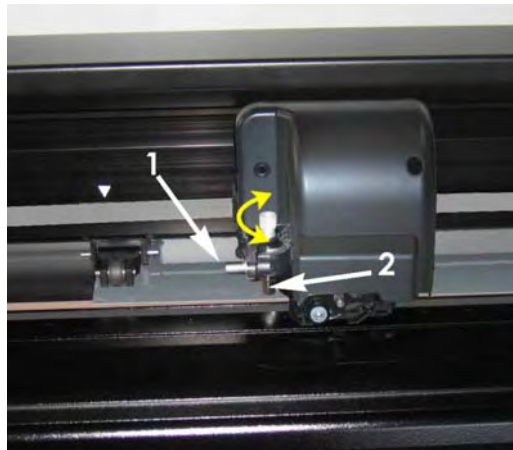
FIG 1-25 REMOVING THE DRAG KNIFE HOLDER FROM THE CLAMP
