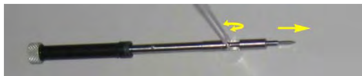
FIG 1-31 REMOVING KNIFE FROM THE TANGENTIAL KNIFE HOLDER
